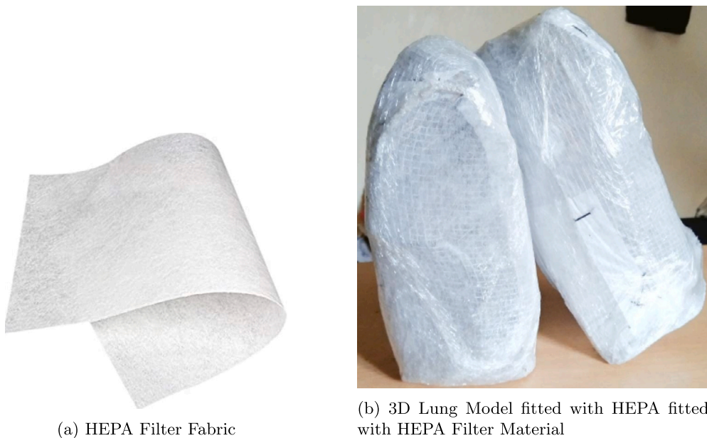
Fig. 6. HEPA Filter Fabric and 3D Lung Model fitted with the HEPA Material.
