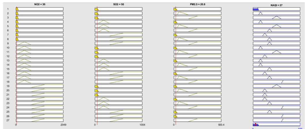
Figure 9. Active rules and Membership functions of input NO 2 , SO 2 , PM 2.5 vs. output of KAQI.
